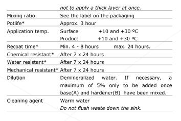
The times and values given are approximate and are affected by fluctuating surface and environmental conditions such as (product)temperature, relative humidity and layer thickness. Ensure good ventilation during curing. Insufficient ventilation will slow down the curing process.
