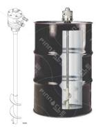
pump. Use a Twistork-helix mixer to obtain a homogeneous mixture. The mixing time depends on the size of packaging. A 200 liter drum, used for the first time or after a longer storage period, should be mixed intensively for 45 minutes. Following this, short and thorough mechanical mixing at every turn is sufficient.
